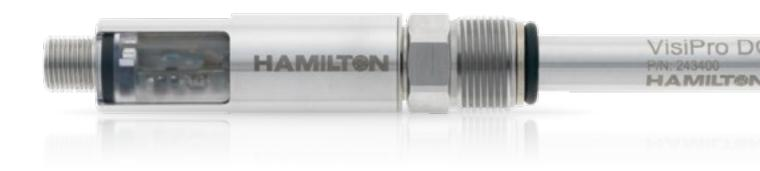
The VisiPro DO is the optical dissolved oxygen (DO) sensor for use in explosive environment. VisiPro DO optical technology improves the measuring performance and simplifies maintenance. Improvements compared to conventional electrochemical (amperometric) sensors include flow independence, rapid startup with no polarization time, and simplified maintenance.
